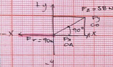
$$\text{Sen } 40^\circ = \frac{F_y}{58 \text{ N}} \rightarrow F_{y1} = 58 \text{ N} \cdot \text{Sen } 40^\circ = 37.28 \text{ N}$$
