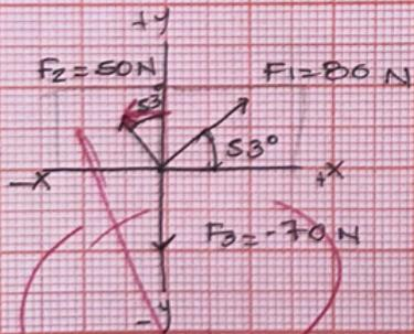
$$3. \Sigma F_y = 63.84 \text{ N} + 30.09 \text{ N} + (-70 \text{ N}) = 23.93 \text{ N} \downarrow$$
