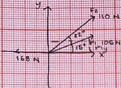
$$\textcircled{1} \cdot \text{Sen } 15^\circ = \frac{F_{1y}}{105 \text{ N}} = 105 \text{ N} (\text{Sen } 15^\circ) = 27.17 \text{ N}$$
