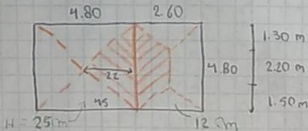
$$\textcircled{1} H_1 = \frac{P}{170} + A \rightarrow \frac{4.80\text{m} + 4.80\text{m} + 4.80\text{m} + 4.80\text{m}}{170} + 0.04\text{m} = 0.152\text{m} = \textcircled{0.25\text{m}}$$
