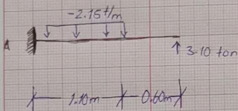
$$P = W \cdot L \rightarrow -2.15 \text{ ton} \cdot 1.10 \text{ m} = -2.365 \text{ ton} \cdot \text{m}$$
