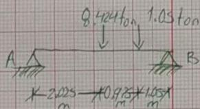
$$M_A = [(-8.424 \text{ ton} \cdot 2.025 \text{ m}) + (-1.05 \text{ ton} \cdot 3.00 \text{ m}) + (R_B \cdot 4.05)] = 0$$
