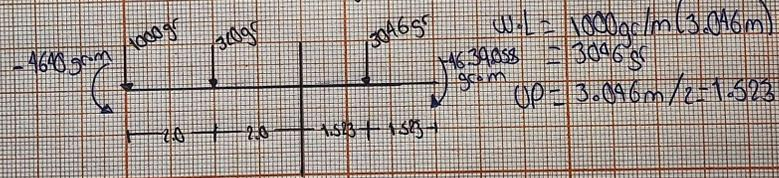
$$3096 \text{ gf} \cdot 1.523 \text{ m} = 4639.058 \text{ gf} \cdot \text{cm}$$
