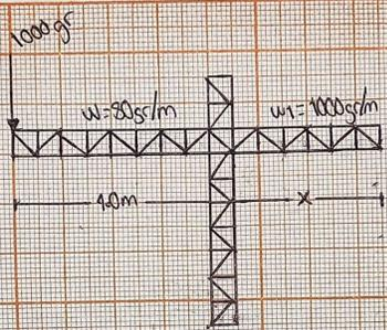
$$w \cdot l = 80 \text{ gf/m} (4.0 \text{ m}) = 320 \text{ gf}$$
