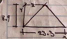
$$I_x = \frac{23.3 \text{ cm} (3.8 \text{ cm}) [(8 \text{ cm})^2 - (8 \text{ cm} \times 23.3 \text{ cm}) + (23.3)^2]}{3} = 29.513 \text{ cm} (64 \text{ cm}^2 - 186.4 \text{ cm}^2 + 542.89 \text{ cm}^2) = 29.513 \text{ cm}^2 (426.49 \text{ cm}^2)$$
