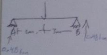
$$P = 0.32 \text{ ton} \cdot \text{m} (6\text{m}) = 0.96 \text{ ton}$$
