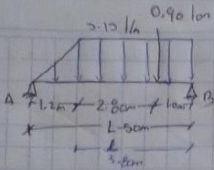
$$P = \left[ \frac{2.0 \text{ m} \cdot 3.80 \text{ m}}{2} \right] \cdot 3.10 \text{ kN/m}$$
