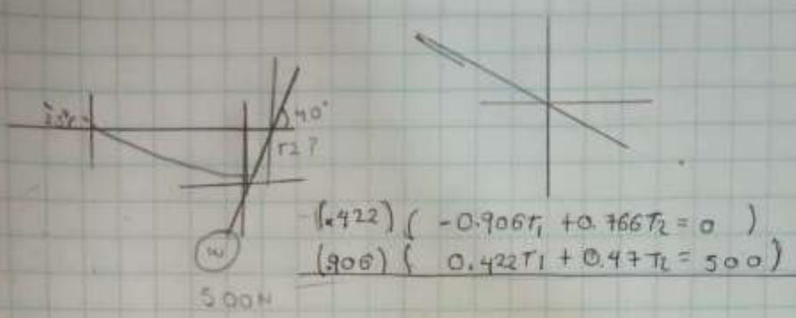
$$\begin{aligned} &(-422) \left( -0.906T_1 + 0.766T_2 = 0 \right) \\ &(900) \left( 0.422T_1 + 0.47T_2 = 500 \right) \end{aligned}$$
