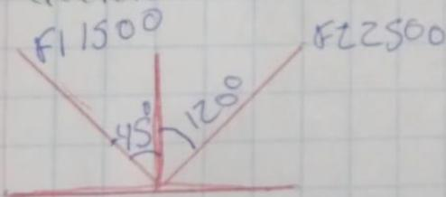
$$\begin{aligned} \Sigma F_X \\ F_1 = 1500 \cos 45^\circ \\ F_2 = 2500 \cos 120^\circ \end{aligned} \left. \vphantom{\begin{aligned} F_1 \\ F_2 \end{aligned}} \right\} \Sigma F_X = -189.34 \text{ N}$$
