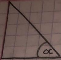
$$\text{Tang } \alpha = \frac{C.O}{C.A} \rightarrow \text{tang}^2 = \frac{18.7619 \text{ kN}}{11.09 \text{ kN}}$$
