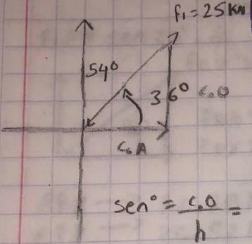
$$\cos \theta = \frac{CA}{h} \Rightarrow \cos 36^\circ = \frac{F_{1x}}{25 \text{ kN}} \rightarrow F_{1x} = 25 \text{ kN} \cdot \cos 36^\circ$$
